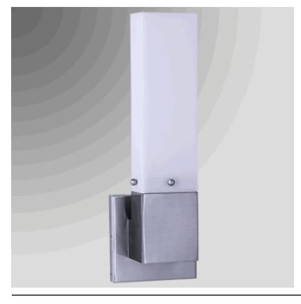
15.25"H Brushed Nickel Wall Sconce, GU24 Socket, direct wired, with White Frosted Acrylic Diffuser perforated at top. Recommend 6 watt LED PL style bulb with GU24 base.
